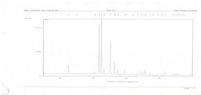
Fig. 6: XRD diffractogram of cefpodoxime proxetil inclusion compound (SF3.3).
