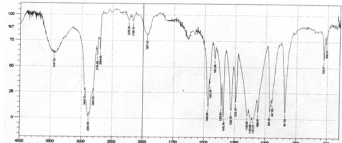
Fig. 3: FTIR spectrum of PVA
