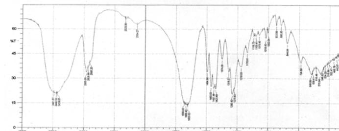
Fig. 2: FTIR spectrum of PVP
