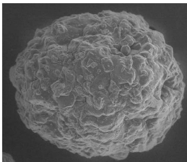
Photograph 1. Scanning electron microscopy of porous microsphere
