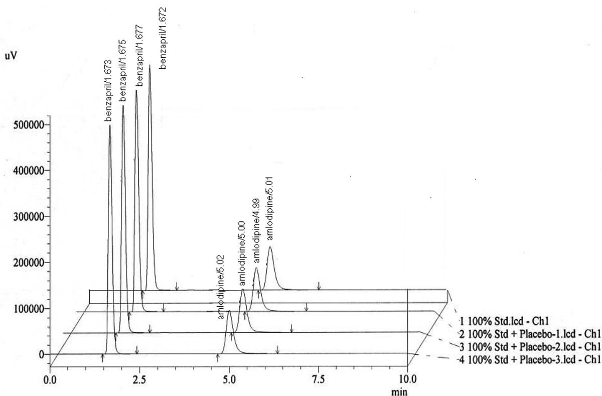
Fig. 2: Chromatogram of benzapril and amlodipine along with 3 placebo formulations.
