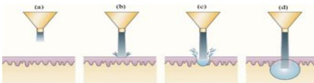
Fig. 5: Schematic of drug delivery using liquid jet injector
