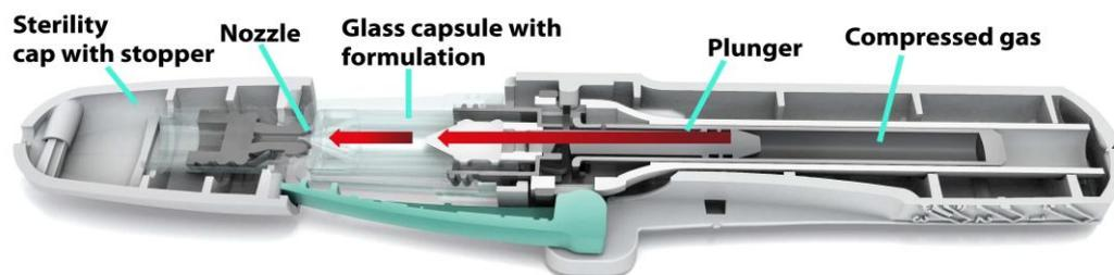
Fig. 3: Design of needle less injection device
