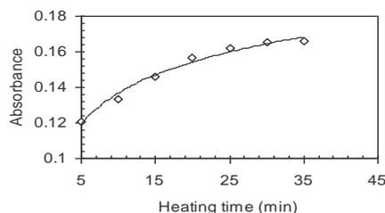
**Fig. 5:** Effect of heating time on iron-cartap complex using cartap (1ml, 1.25 mg/ml), alkaline hydroxylamine (5 M), hydrochloric acid (6 M), ferric chloride (0.5 M) and temperature (70°C) at 542 nm.
