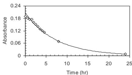
**Fig. 6:** Stability of the complex color using cartap (1ml, 1.25 mg/ml), alkaline hydroxylamine (5 M), hydrochloric acid (6 M), ferric chloride (0.5 M) and temperature (70°C) at 542 nm.
