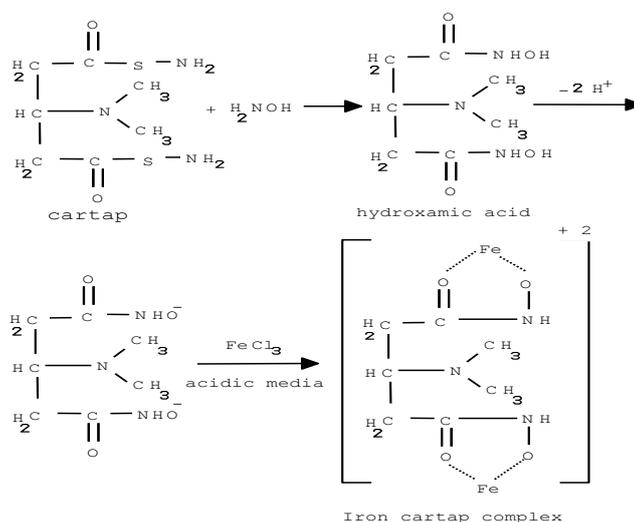
**Scheme 1: Possible mechanism of the reaction.**
