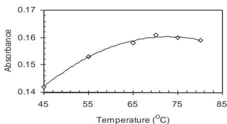
**Fig. 4:** Effect of Temperature on iron-cartap complex using cartap (1ml, 1.25 mg/ml), alkaline hydroxylamine (5 M), hydrochloric acid (6 M) and ferric chloride (0.5 M) at 542 nm for 25 min
