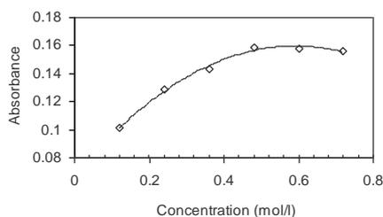
**Fig. 2:** Effect of hydrochloric acid on iron-cartap complex using cartap (1ml, 1.25 mg/ml), alkaline hydroxylamine (5 M), ferric chloride (0.5 M) and temperature (70°C) at 542 nm for 25 min.
