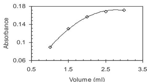
**Fig. 1: Effect of alkaline hydroxylamine on iron-cartap complex using cartap (1ml, 1.25 mg/ml), hydrochloric acid (6 M), ferric chloride (0.5 M) and temperature (70°C) at 542 nm for 25 min**
