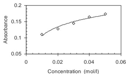
**Fig. 3:** Effect of ferric chloride on iron-cartap complex using cartap (1ml, 1.25 mg/ml), alkaline hydroxylamine (5 M), hydrochloric acid (6 M) and temperature (70°C) at 542 nm for 25 min.
