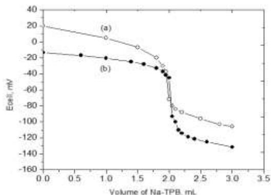
**Fig. 5: Potentiometric titration of 6.90 mg FXCl against  $10^{-2}$  mol/L Na-TPB using a) FX-PM and b) FX-TPB carbon paste electrodes.**
