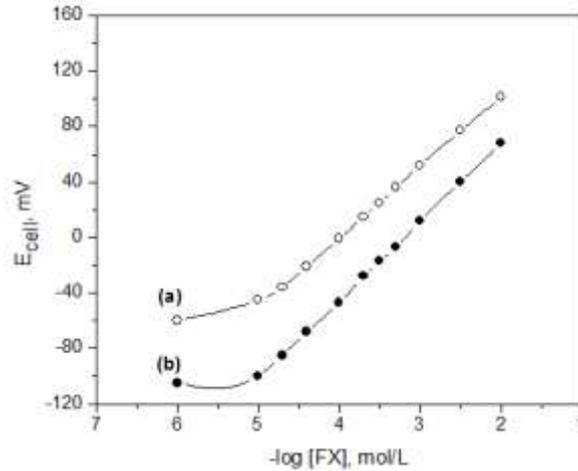
Fig. 1: Calibration curve of a) FX-PM and b) FX-TPB carbon paste electrodes.
