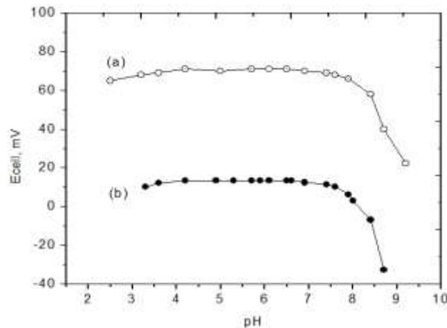
Fig. 2: Effect of pH change of  $10^{-3}$  mol/L FXCl solution using a) FX-PM and b) Na-TPB based carbon paste electrodes.
