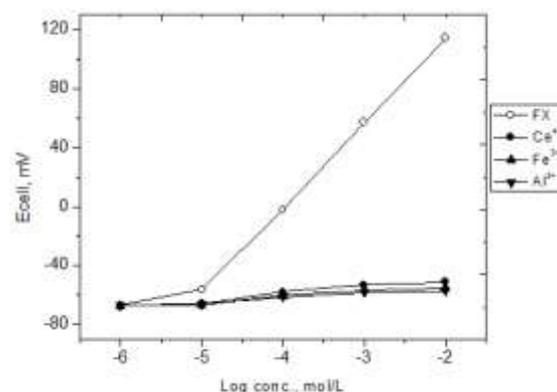
Fig. 4:  $E_{cell}$ -logc curves for determining the MPM selectivity coefficient of FX-PM carbon paste electrodes for FXCl against  $Al^{3+}$ ,  $Fe^{3+}$  and  $Cr^{4+}$ . The initial reference solution of FXCl was  $1 \times 10^{-6}$  mol/L.
