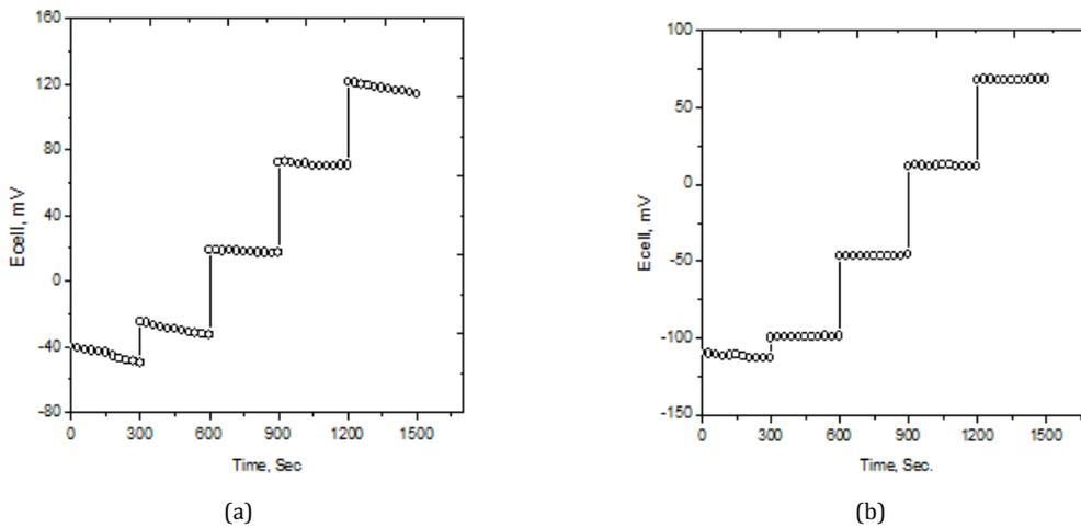
Fig. 1: Typical potential-time plot for the response of a) FX-PM and b) FX-TPB carbon paste electrodes.
